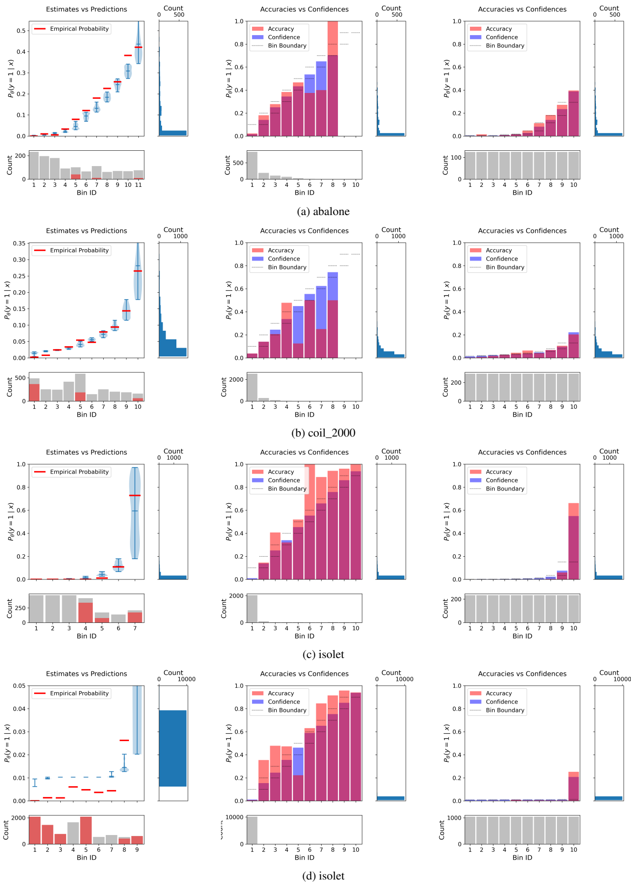
Figure 6: Comparison of visual representations of TCE, ECE and ACE for the logistic regression algorithm. (Left) The test-based reliability diagram of TCE. (Middle) The reliability diagram of ECE. (Right) The reliability diagram of ACE. Each row corresponds to a result on the dataset: (a) abalone, (b) coil_2000, (c) isolet, and (d) webpage.
