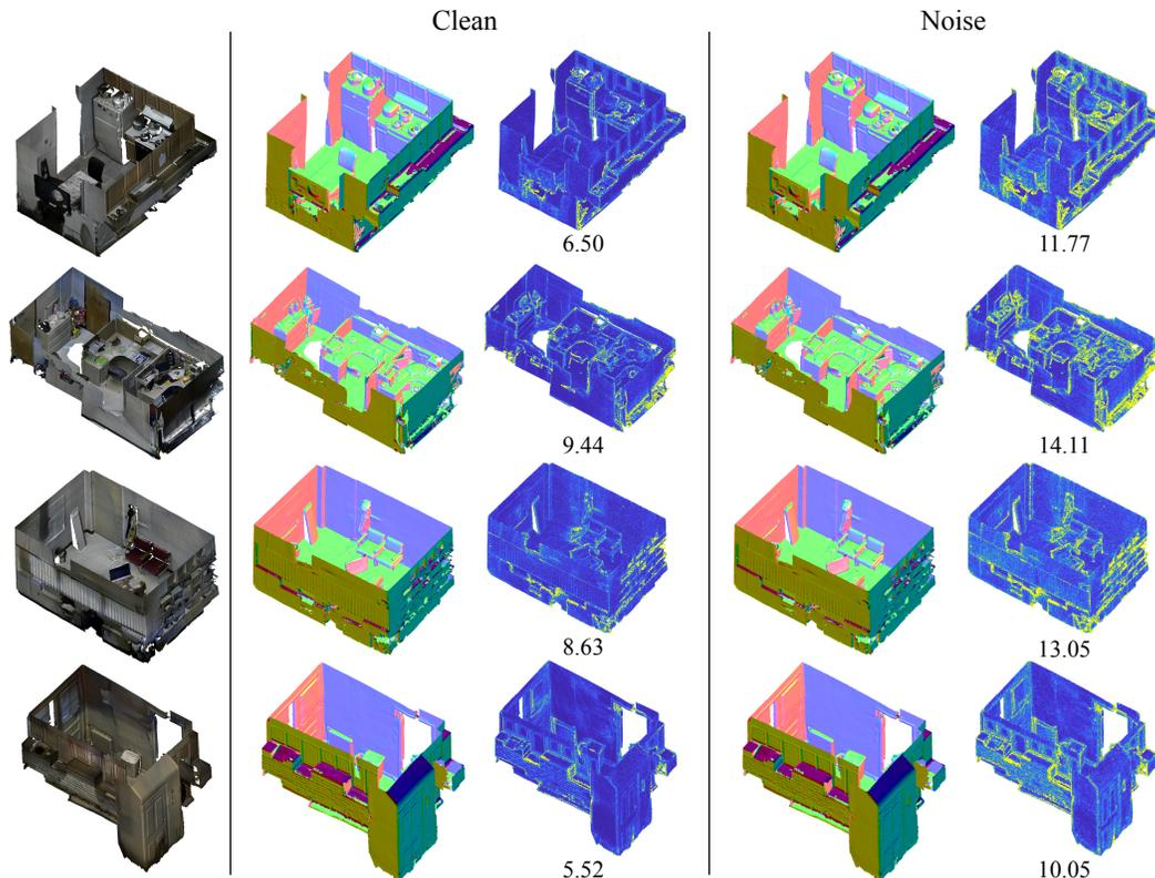
Figure 6: Visualization of the SceneNN dataset [9] and our estimated point normals. The first column is the 3D point clouds with RGB colors of real-world indoor scenes. The columns 2 and 4 are point normal vectors mapped to RGB. The columns 3 and 5 are point normal angular errors mapped to a heatmap ranging from 0-16 degrees. The number under the point cloud is its RMSE.
