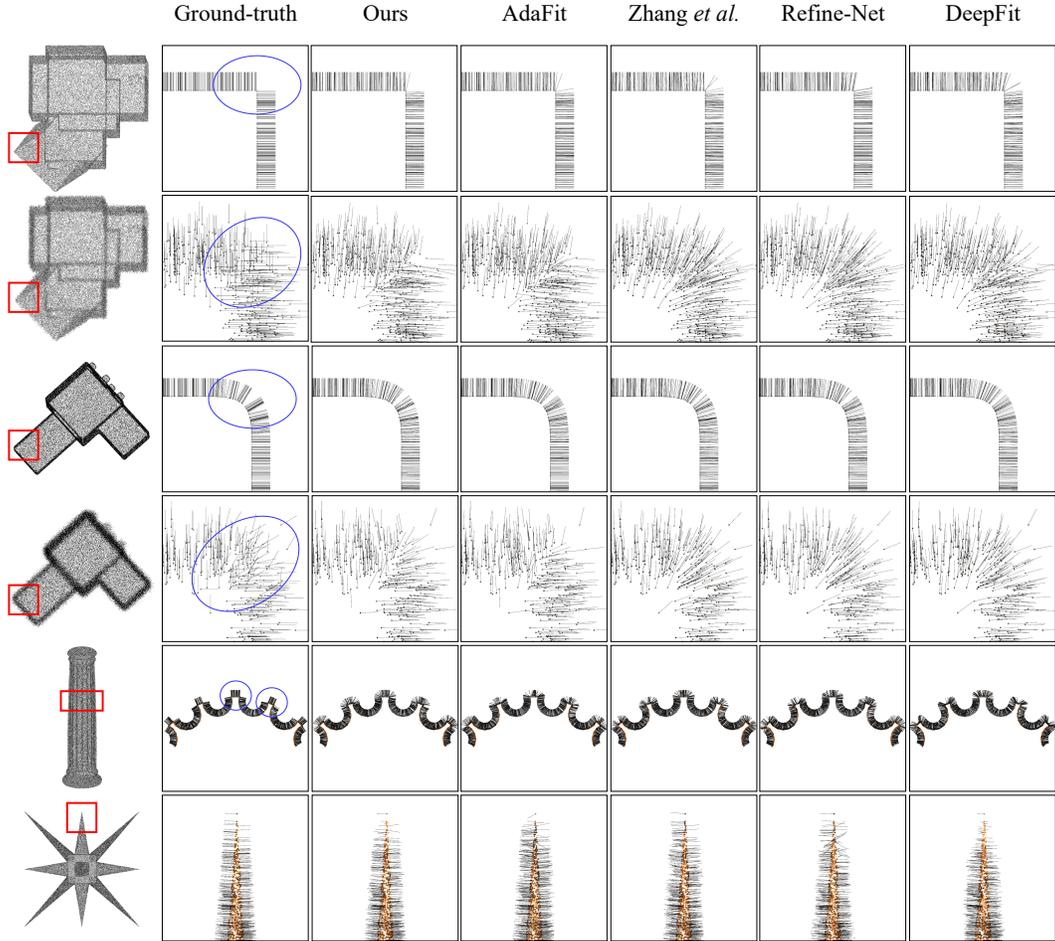
Figure 2: Cutting plane visualization of the estimated normals (black lines) in different regions with complex geometric structures.
