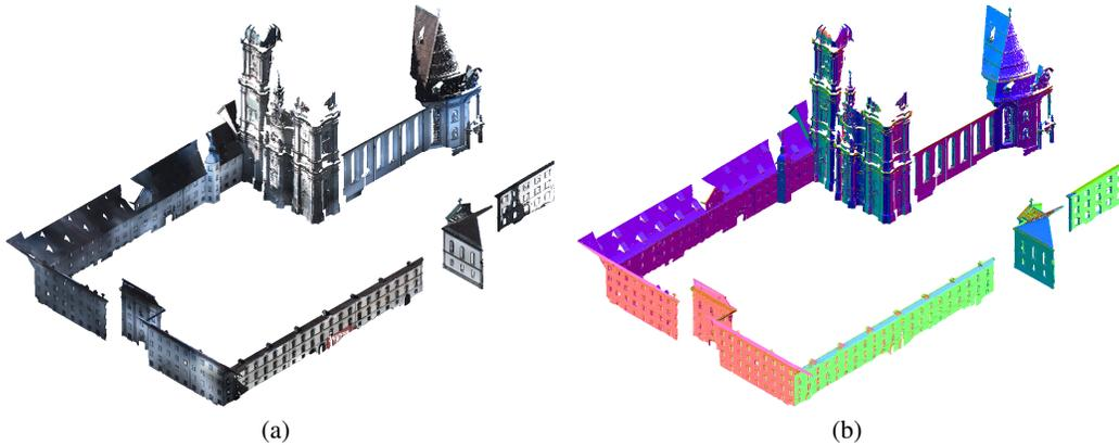
Figure 5: Visualization of the Semantic3D dataset [7] and our estimated point normals. (a) The raw 3D point cloud with RGB colors of the real-world outdoor scene. (b) Our estimated point normal vectors mapped to RGB.
