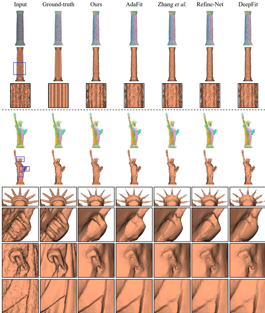
Figure 3: Qualitative comparison results of point cloud filtering using the estimated normals of different methods. The input and filtered point clouds are shown with RGB colors, and their corresponding reconstructed shape models are provided under each point cloud. The local enlarged views are provided under each shape.
