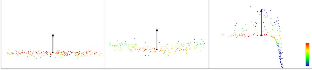
Figure 1: Visualization of the contribution of each 3D point to estimate the normal of the query point (black). The red points are weighted higher than the blue points.
