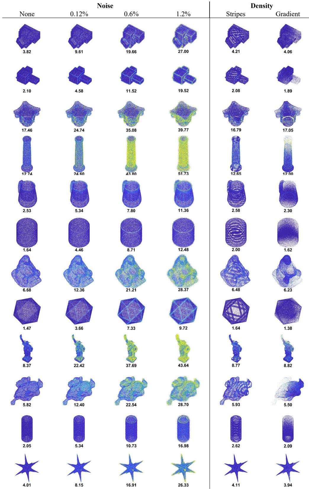
Figure 8: Error visualization for different noise levels and density variations of the PCPNet dataset [6]. The point color is the angular error mapped to a heatmap ranging from 0-40 degrees.
