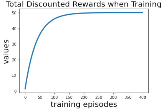
Figure 7: The total discounted rewards converges to the optimal value after about 280 training episodes.
