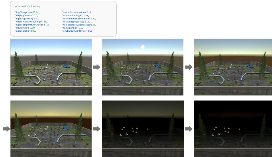
Figure 17: Day/night cycle configuration and visual transition examples. Top: Configuration parameters controlling the day-night cycle, including fog density, temperature shift, sun angle, and clipping distance. Bottom: Five key visual phases of the cycle: day, sunset, night, deepnight, and dawn. These phases dynamically modulate ambient lighting, visibility, and temperature, influencing agent behavior and sensory inputs.
