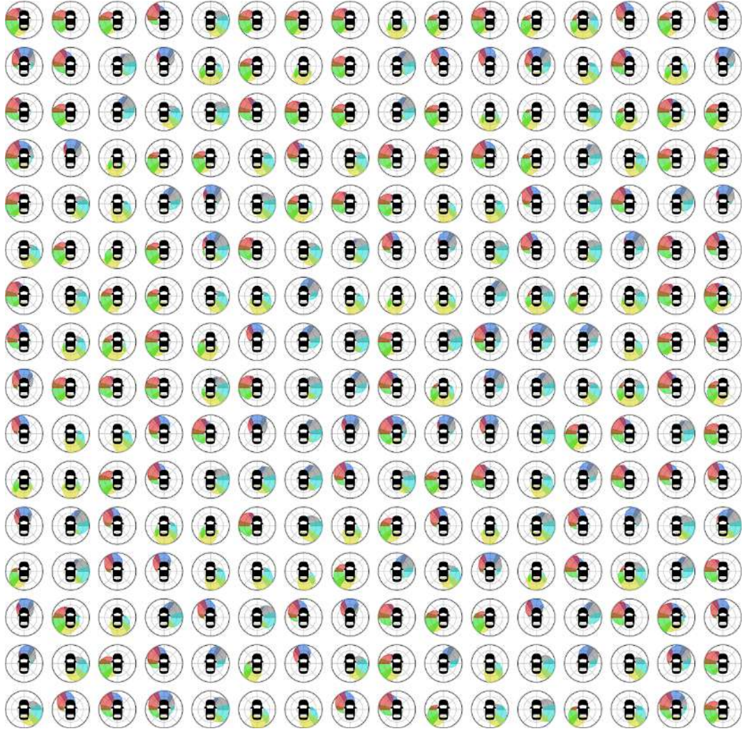
Figure 12: Input-to-latent attention study — all the latent vectors for an attention head. These polar plots represent the directional attention intensity of the 256 latent vectors for a randomly chosen attention head (head #4). As shown in Figure 9, one attention head generally covers the full scene over the latent vectors.
