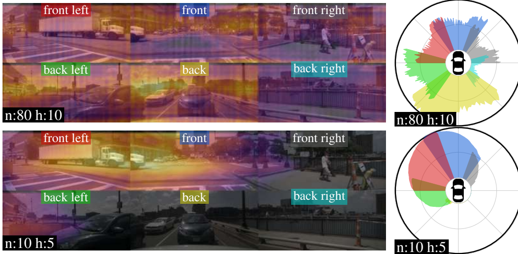
Figure 6: Input-to-latent attention study. Analysis of attention maps for two networks trained with different input embeddings. Top row is with ‘Fourier + Cam. idx’ and bottom row is with our proposed ‘Cam. rays’ embedding. The attention for one attention head and one latent is shown on the left superimposed with RGB images. The polar plots represent the directional attention intensity for one attention head with one latent vector. The radial distance is proportional to the attention level and shows the directions the network attends to the most.
