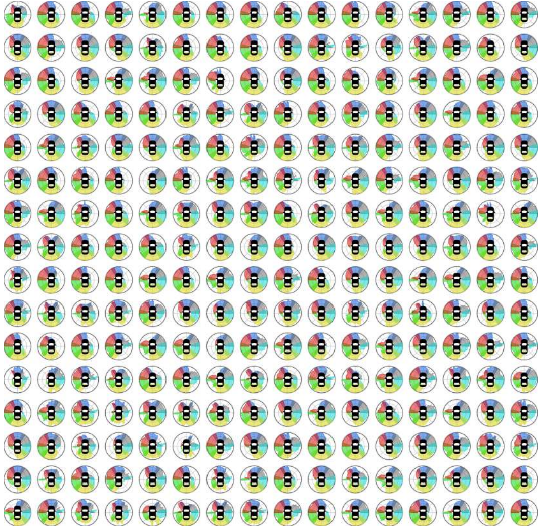
Figure 10: Input-to-latent attention study — average over heads. These polar plots represent the directional attention intensity averaged over all attention heads for the 32 attention heads. When averaging over attention heads, we observe that the average attention spans over half of the scene. This allows latent vectors to extract long-range context between views with the capacity to disambiguate them.
