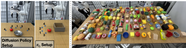
Fig. 2: Left : Evaluation setup illustrating pick object initial conditions. Right : Objects used for real-world and paired simulation evaluations.
