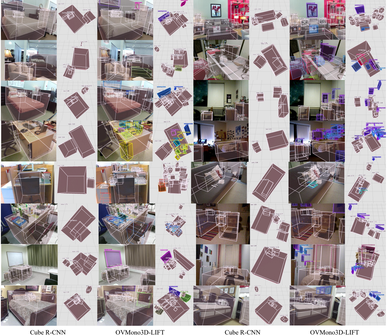
Figure 9. Qualitative Visualizations on the SUN RGB-D [59] Test Set. For each example, we present the predictions of Cube R-CNN [3] and OVMONO3D-LIFT, displaying both the 3D predictions overlaid on the image and a top-down view with a base grid of 1\text{ m} \times 1\text{ m} tiles. Base categories are depicted with brown cubes, while novel categories are represented in other colors.
