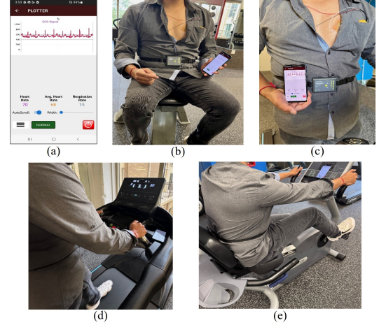
Fig. 3. Experimental protocol and data collection setup. (a) Real-time CardioHelp app visualization; (b) Sitting with the custom wearable device, ECG electrodes, and reference respiration belt; (c) Walking at 2 mph and (d) running at 3 mph on a treadmill; (e) Stationary cycling at 6-7 mph.
