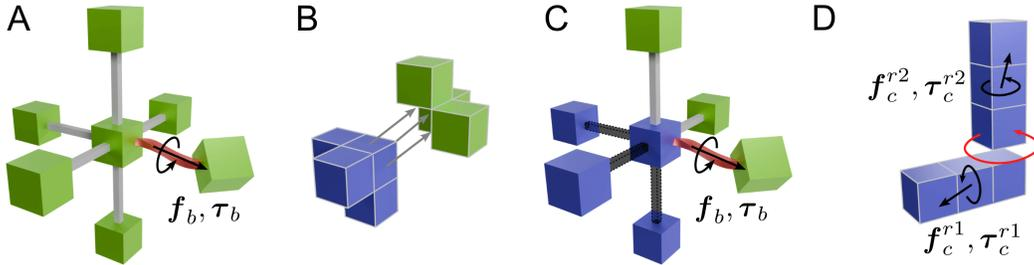
Figure 4: **Simulating endoskeletal robots.** Soft tissues (green masses) were modeled by a grid of Euler–Bernoulli beams (A) that may twist and stretch and directly attach to bones (blue masses; B and C) that follow rigid bodied dynamics with joint constraints (D). More details about the simulator can be found in Sect. 2.1 and Appx. B.
