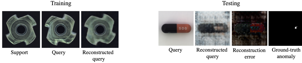
Figure C: Applying the proposed adaptive sparse coding layer to an auto-encoder for few-shot anomaly detection and localization suffers severely from the poor generalization of the decoder, which delivers consistently high reconstruction error on novel tasks.
