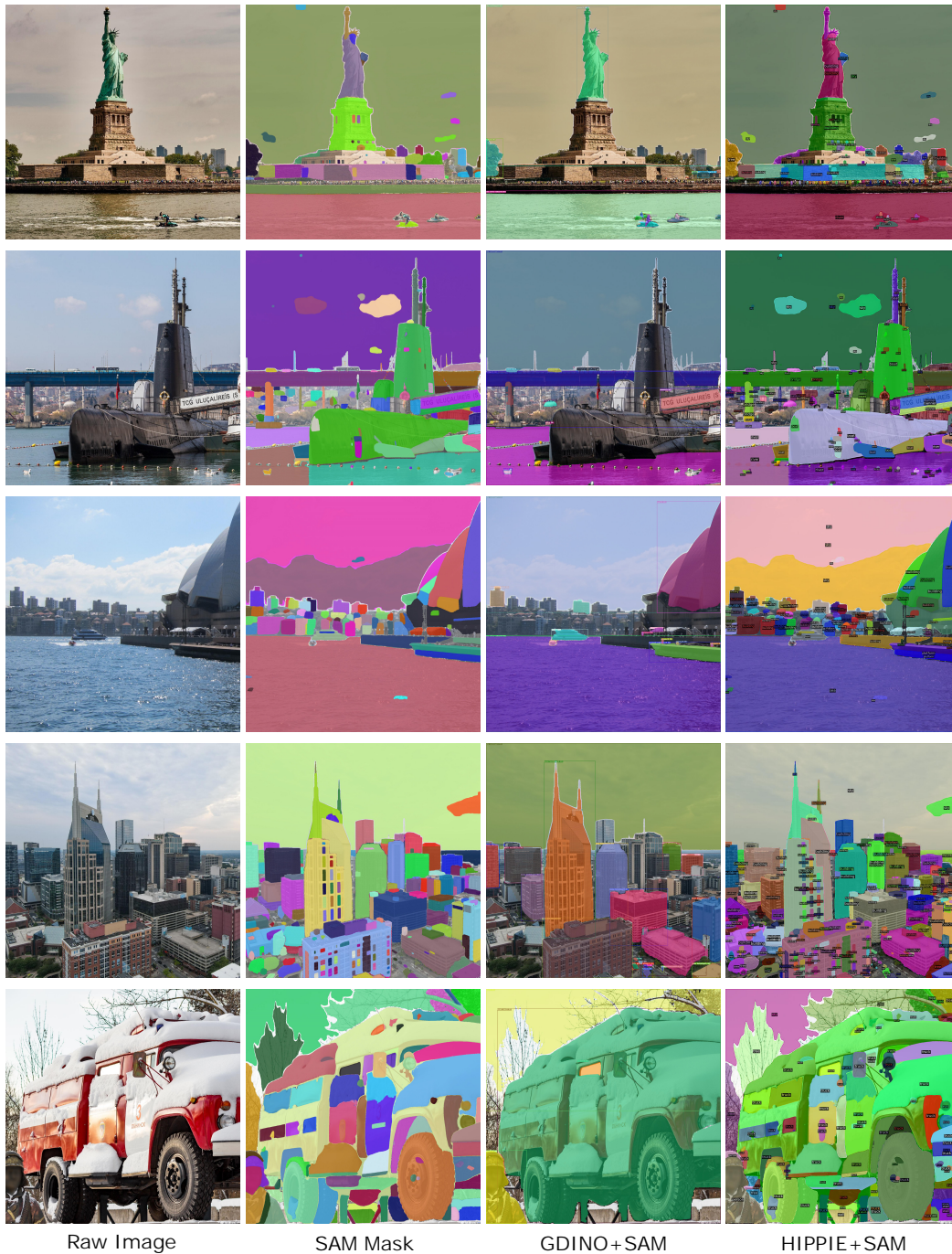
Figure A7: Additional results of merging HIPIE with SAM for hierarchical segmentation. By integrating the part masks from our model and conducting a vote among SAM’s panoptic masks, we generate finely detailed mask outputs. Our method demonstrates fewer misclassifications and overlooked masks across the SA-1B dataset compared to the Grounding DINO + SAM approach. Furthermore, our technique excels in differentiating between intra-class objects and identifying distinct object parts.
