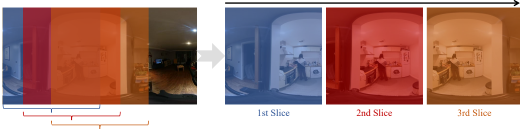
Figure 4: The illustration of the projection process from a 360° image to horizontal slices.
