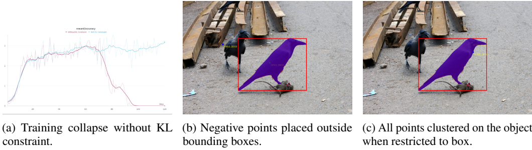
Figure 4: Ablation study failures: (a) Removing the KL constraint leads to training instability and collapse. (b) Encouraging both positive and negative point generation causes negatives to appear outside target areas. (c) Forcing all points into the bounding box eliminates useful contrast, reducing performance.
