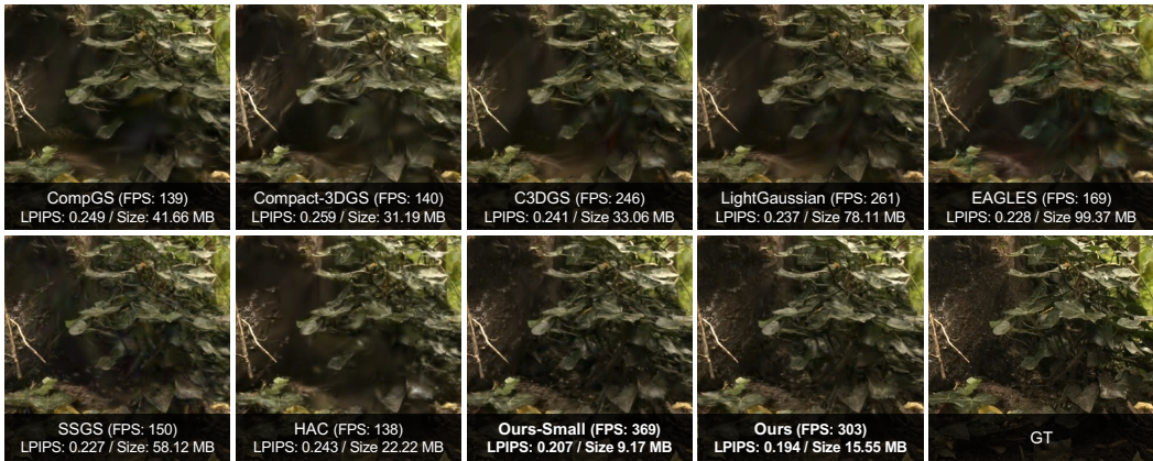
Figure 5: Qualitative results on the ‘stump’ scene of Mip-NeRF 360 (Barron et al., 2022). Rendering speed, LPIPS, and storage size are shown at the bottom of each subfigure.
