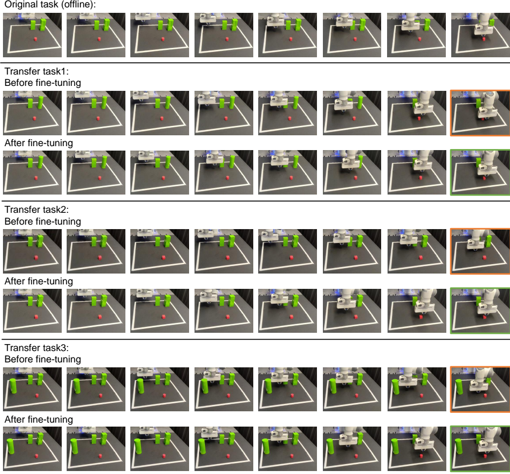
Figure 10. Deployment on different real-world unseen tasks. The trails from top to bottom show the original offline training task and three unseen fine-tuning tasks, with each fine-tuning task displaying both before and after fine-tuning trails. The green frames indicate successful task completion, while the orange frames represent failures.
