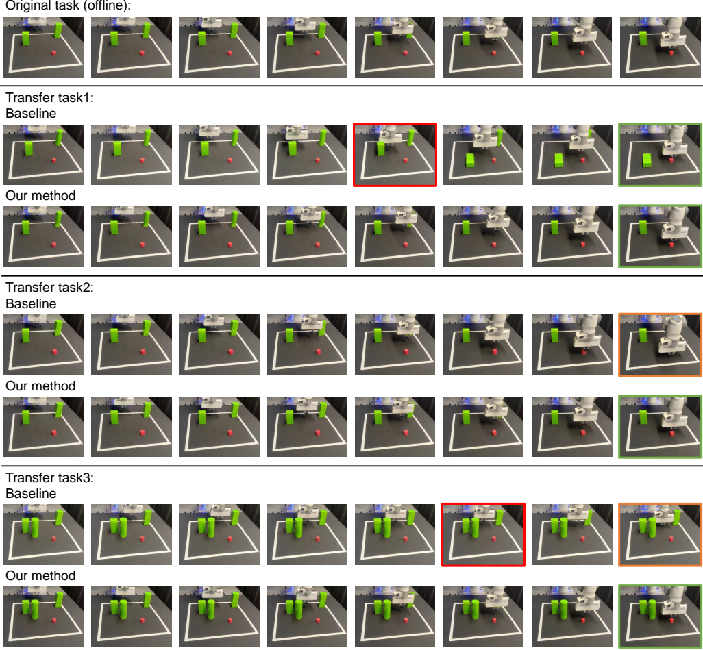
Figure 11. Compare with baseline on different real-world unseen tasks. In each task, we compare our method with the fine-tuned SafeDreamer (baseline). The green frames indicate successful goal reaching, the red frames indicate constraint violations and the orange frames represent failures.
