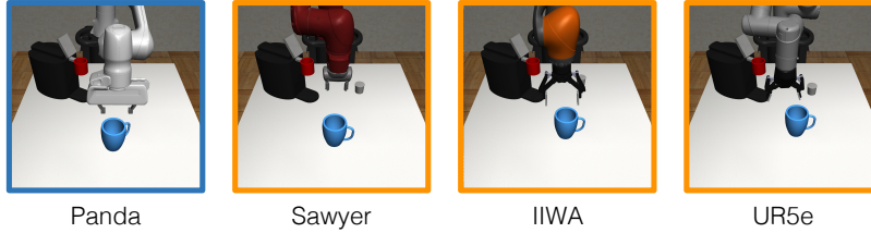
Figure E.1: Robots used in Robot Transfer Experiment. The figure shows the robot arms used for data generation. Source datasets were collected on the Panda arm (blue border) and used to generate data for the Sawyer, IIWA, and UR5e arms (orange border).
