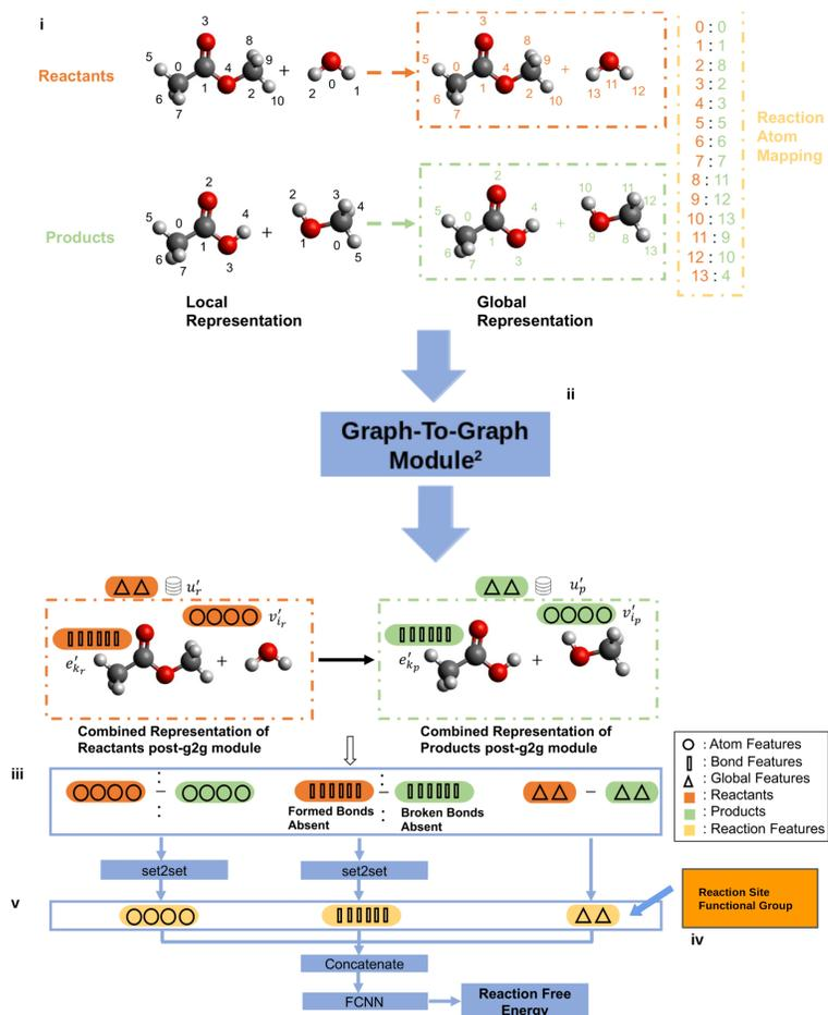
Figure S4: The user inputs atom-mapped sets of reactants and products (i) which undergo message-passing and update steps (ii). Using the user-specified mappings, these updated features are mapped to a global reaction graph (iii) where functional groups at the reaction site are added as global features (iv). Embeddings of bond and atom features plus global features directly serve as the fixed-size vector used in a conventional dense neural network for property prediction.
