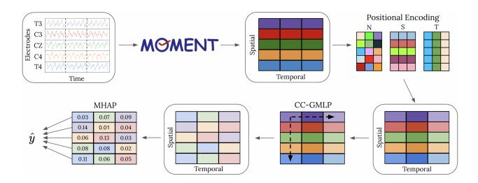
Figure 1: A diagram showing how EEG data is processed by MOMENT and STAMP. The EEG data is separated into tokens, which are embedded using MOMENT before positional encoding is applied. The resulting tokens are passed through the CC-GMLP, where spatial and temporal relationships are incorporated into embeddings. MHAP then determines relevant features and generates final predictions by projecting embeddings into lower dimensional spaces.
