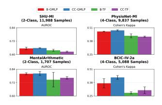
Figure 3: Performance comparison between four different token mixer options: B-GMLP (0.79M), CC-GMLP (0.74M), B-TF (1.25M), and CC-TF (0.99M). The value in parentheses indicates the average number of trainable parameters across the 4 datasets.
