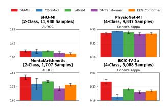
Figure 5: Performance comparison between the full evaluation of 5 methods: STAMP (0.74M), CBraMod (29M), LaBraM (5.8M), ST-Transformer (3.5M), and EEG Conformer (0.55M). The value in parentheses indicates the average number of trainable parameters across the 4 datasets.
