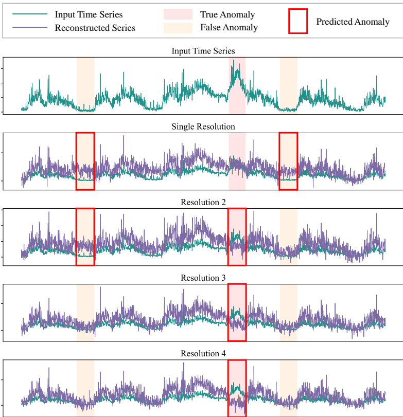
Figure 7: Comparison of detection performance across different resolution settings originates from the SMD dataset, where the pink and yellow areas represent true anomalies and false anomalies (normal data), respectively. The green and purple lines indicate the input time series and the reconstructed time series, respectively, while the red bold frame highlights anomalies detected by the model.
