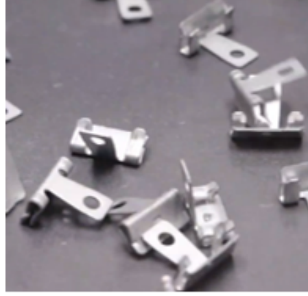
Figure 8: the objects considered, metallic hinges from the automotive sector (De Paola et al., 2024).
