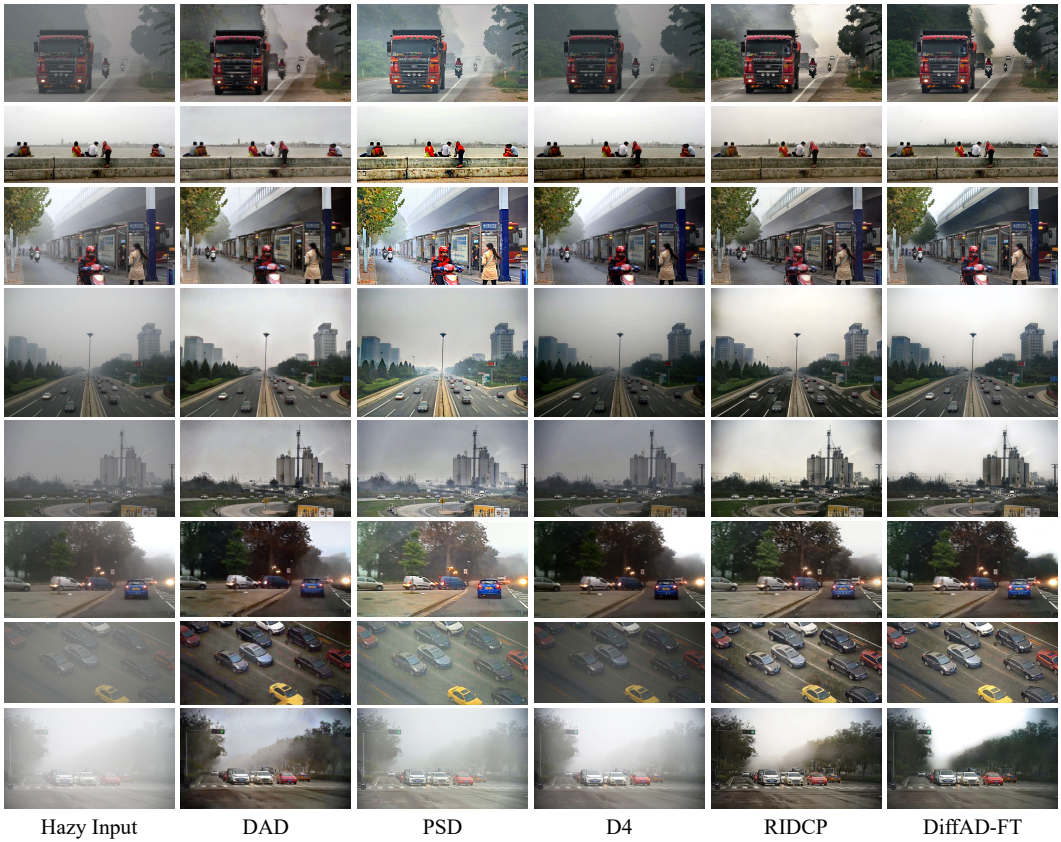
Figure 18: Dehazing results of various methods on RTTS dataset. Please zoom in on screen for a better view.
