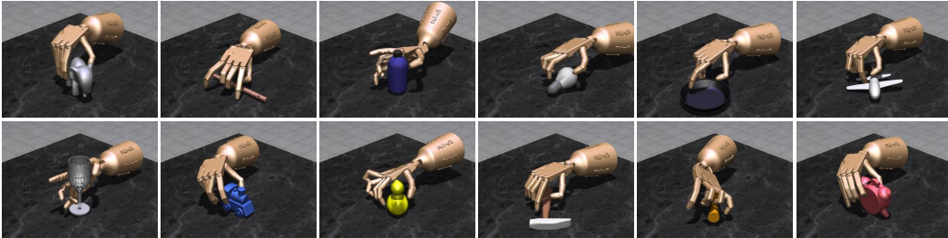
Figure 7: Examples of pre-grasps used in our experiments. Note how they (1) place the hand in proximity to the target object and (2) pose the fingers around functional parts of the object (e.g. hammer’s handle). However, pre-grasps are not stable grasps. In fact, the hand does not make contact with the objects at all!
