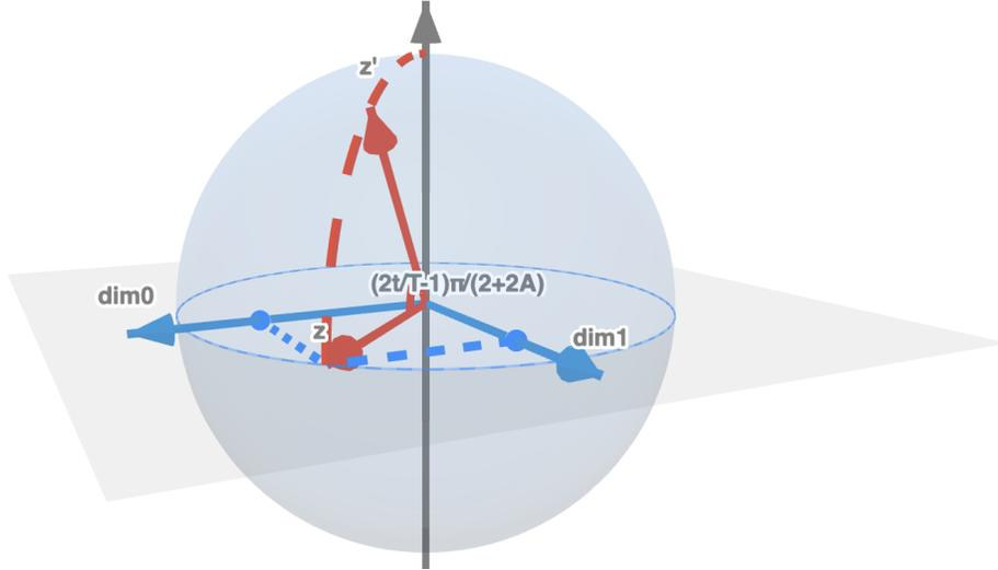
Figure 6: An example of our time-step embedding method. Here we use an example of 2 dimension  $z = (x, y)$ . When  $z$  is at time-step  $t$ , the embedded feature vector is  $z' = \left( \sin \frac{(2t/T - 1)\pi}{2 + 2A}, x \cos \frac{(2t/T - 1)\pi}{2 + 2A}, y \cos \frac{(2t/T - 1)\pi}{2 + 2A} \right)$ .
