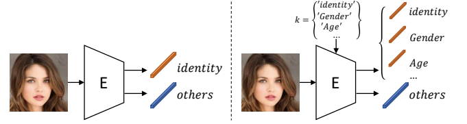
Figure 2: Differences between existing disentanglement method for anonymization (left) and our solution (right). E denotes the disentanglement network.
