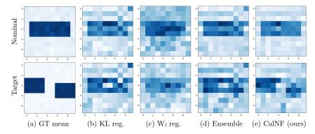
Figure 3: **Seismic waveform inversion.** (a) The ground truth nominal and target density profiles. (b-d) The posteriors fit using KL and  $W_2$  regularization and CALNF (ours is the only method able to correctly infer the target density profile).
