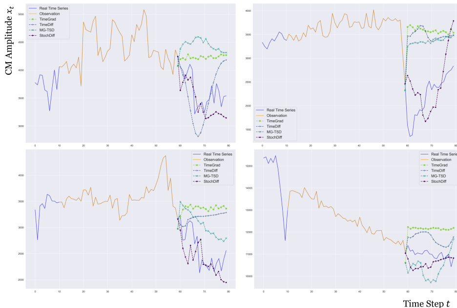
Figure 3: Cochlear Implant Forecasting Simulations. The blue line is the real CM amplitude, and the orange part is the observation that was fed to the model. Forecasting from different models are marked with differently according to the legend inside the plots.
