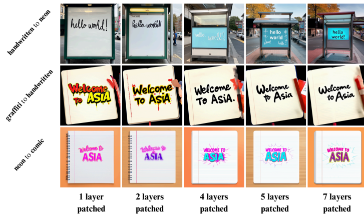
Figure 14: The style of the text in Stable Diffusion 3 is influenced by at least 7 layers. We provide results demonstrating performance in editing textual style when patching an increasing number of layers in the diffusion model. Although modifying this feature becomes feasible with 7 layers, it significantly alters the image background as well.
