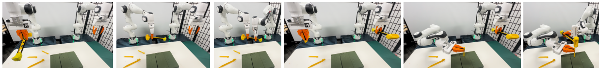
Fig. 1. Long-horizon task with inter-step dependencies. The goal of the task above is to hammer the nail into the board. A successful trajectory must handover the hammer to the right arm and both arms must coordinate to strike the nail. Compositional generative sampling can solve such tasks using only atomic skill level demonstrations and without any task-level demonstrations.
