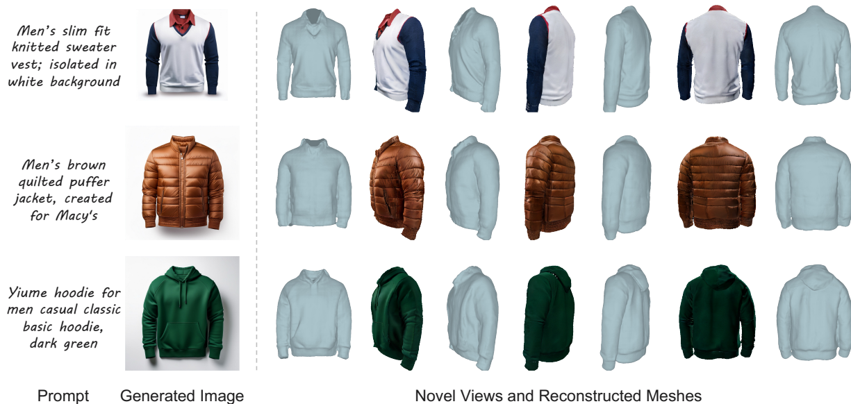
Figure S9. Compatibility with generative apparel. By reconstructing both geometry and texture from synthetic garment images, GarmentCrafter demonstrates its adaptability to AI-generated designs. The results showcase the ability of GarmentCrafter to handle diverse and complex inputs, expanding its potential applications to generative fashion and virtual apparel workflows.
