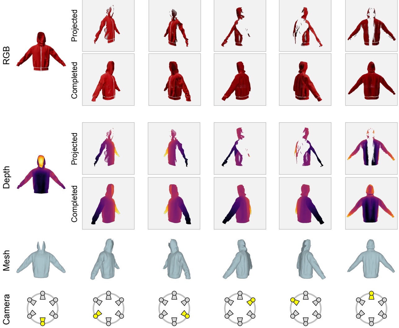
Figure S2. Intermediate results of progressive novel view synthesis along a full camera trajectory. From an input RGB image (top-left), GarmentCrafter progressively synthesizes novel view RGB and depth maps following a zigzag camera trajectory.
