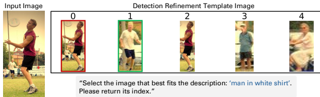
Figure 2. Detection Refinement Example. Starting with candidate detections from GroundingDINO [10], we select the top k predictions and present them as a grid of cropped images (right). We then query the VLM to return the index that best aligns with the input text prompt. Red indicates GroundingDINO’s initial choice and green indicates the refined choice.
