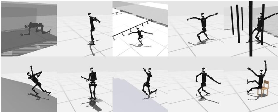
Figure 12: **HumanoidBench locomotion suite visualization.** Images of the Unitree robot we control in the HumanoidBench locomotion suite. The tasks include running, walking, crawling, balancing, sitting, reaching, and performing actions like walking on stairs or walking while avoiding collisions with poles, which cover a diverse range of robotic locomotion scenarios.
