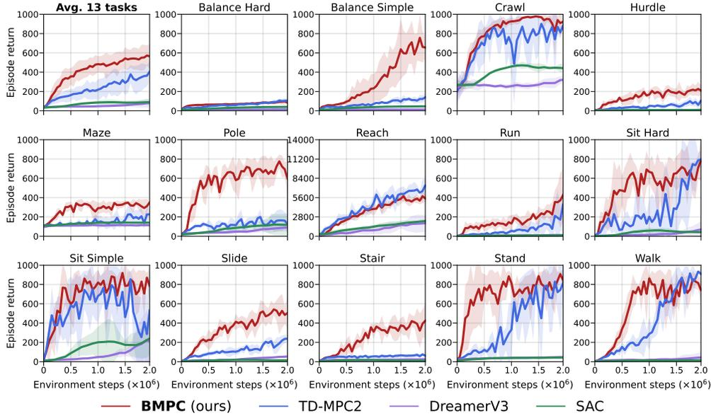
Figure 5: **HumanoidBench locomotion suite.** Comparing BMPC to baselines on HumanoidBench locomotion suite. In the top left, we present the average performance of all 13 tasks except for Reach due to the different reward scales. Mean and 95% CIs over 5 seeds.
