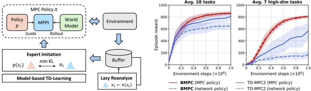
Figure 1: **Overview.** (left) BMPC learns a network policy through expert imitation and lazy reanalyze mechanism, planning during inference using guided MPC, and performs model-based value learning in an on-policy manner. (right) Averaged evaluation performance of the network policy compared to the MPC policy in BMPC and TD-MPC2 on DMControl tasks. BMPC achieves better policy learning, which further boosts the performance of MPC. Mean and 95% CIs over 5 seeds.
