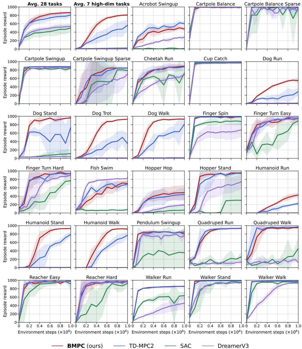
Figure 9: **All DMControl tasks.** Comparing BMPC to baselines on DMControl tasks. In the top left, we present the average performance of 7 high-dimensional locomotion tasks and all 28 tasks. Mean and 95% CIs over 5 seeds<sup>7</sup>.
