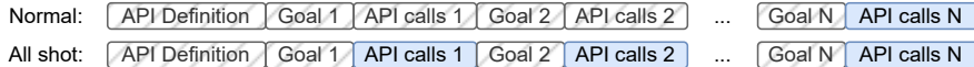
Figure 6: We use all-shot loss for model alignment. We concatenate several examples into a single training sample and backpropagate through the loss on the blue actions in every example. There is no separator token between examples.
