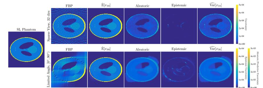
Fig. 1: The reconstructions for sparse view CT with 32 directions (top) and limited angle with  $[0, 90^\circ]$  (bottom).
