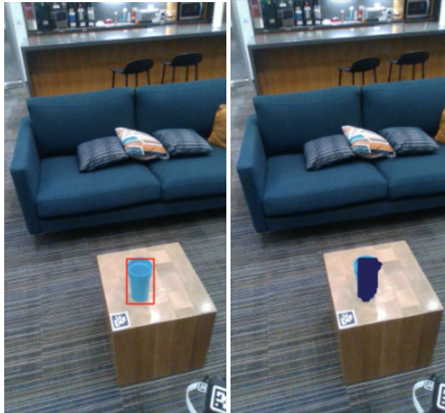
Figure 1: The robot detects and localizes the cup using YOLO-World and segments the result with FastSAM on a frame captured from its head camera for perception.
