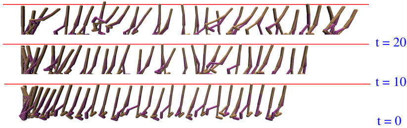
Figure 3: Walker2D planning denoising diffusion with the robust-safe diffuser (Up to down: diffusion time steps 20, 10, 0, respectively). The red line denotes the roof the walker needs to safely avoid during locomotion (safety specifications). Safety is violated at step 20 since the trajectory is initially Gaussian noise, but is eventually guaranteed (step 0). Note that the robot top could touch the roof, and this is not a collision. This can be avoided by defining a more strict safety constraint.
