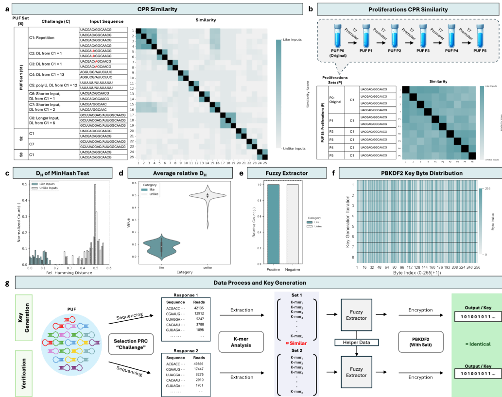
Figure 4: Verification and Key Generation Process using RNA-based PUFs Workflow
