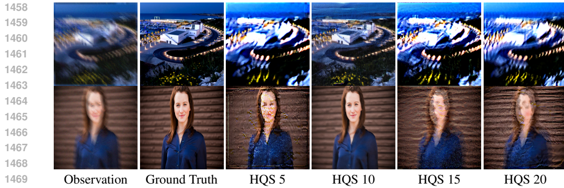
1471 Figure 17: HQS times cause divergence. If the HQS times are not chosen carefully, it will lead to 1472 divergence results.
