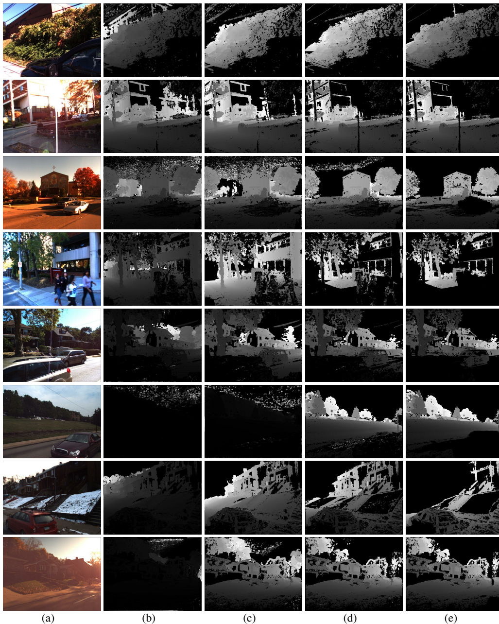
Figure 1: The processing samples given RGB image followed by normalized depth maps for clear visualization of (a) dense reconstruction, (b) range filtering, (c) HSV-based refinement and (d) manual post-processing.
