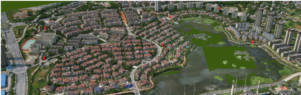
Figure 2: When capturing raw aerial images with a UAV, the positions of ground control points are manually set by the personnel on the ground.
