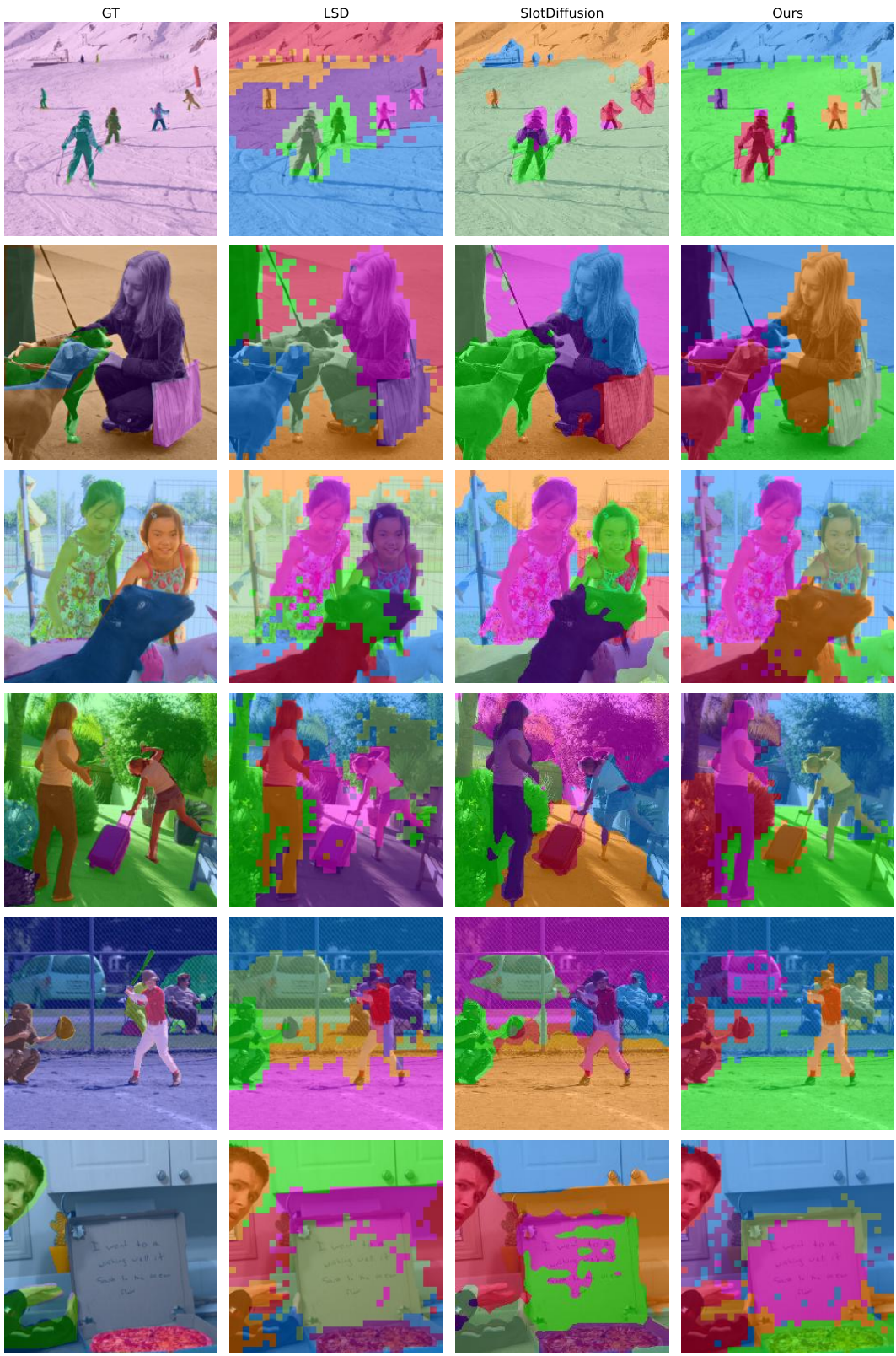
Figure 11: Segmentation comparisons with other methods We show visualizations of predicted segments on COCO dataset. Compared to other models, our model predicts more complete masks without segmenting objects into parts.
