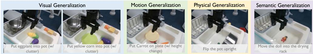
Figure 13: Illustration of tasks used in the WidowX pick-and-place experiments. The selected tasks evaluate different aspects of generalization—Visual, Motion, Physical, and Semantic—following the setup in OpenVLA (Kim et al.).
