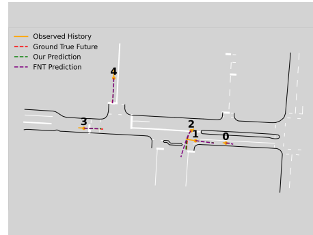
(f) The FNT model failed to predict the slow movement of v_1 and thus wrongly predicted v_2 as making ag-gressive and dangerous movement while the proposed model made the correct prediction for both v_1 and v_2 .
