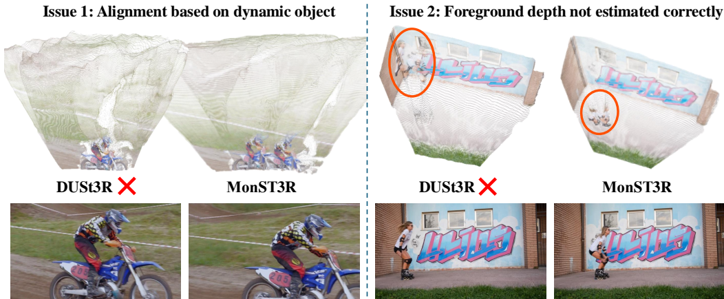
Figure 2: Limitation of DUS3R on dynamic scenes. Left: DUS3R aligns the moving foreground subject and misaligns the background points as it is only trained on static scenes. Right: DUS3R fails to estimate the depth of a foreground subject, placing it in the background.
