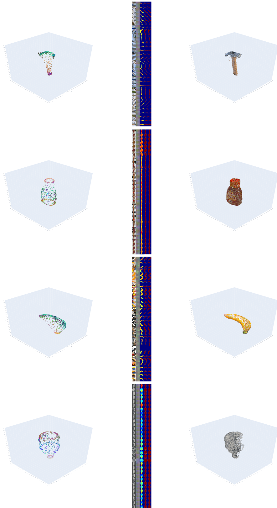
Figure 9. NeMOs from benchmark objects. We show the NeMOs (left, with PCA feature visualization), dense predictions (middle) and object surface reconstruction (right) from objects selected from different datasets. From top to bottom, the datasets are: HANDAL, HOPEv2, YCB-V and T-LESS. We use 32 template images to generate the NeMOs and use the same 32 images to show the dense prediction results. Note that we show real template images for HANDAL, HOPEv2 and YCB-V and synthetic template images for the T-LESS object. All NeMOs have been aligned with the ground truth pose as described in Sec. 7.4.
