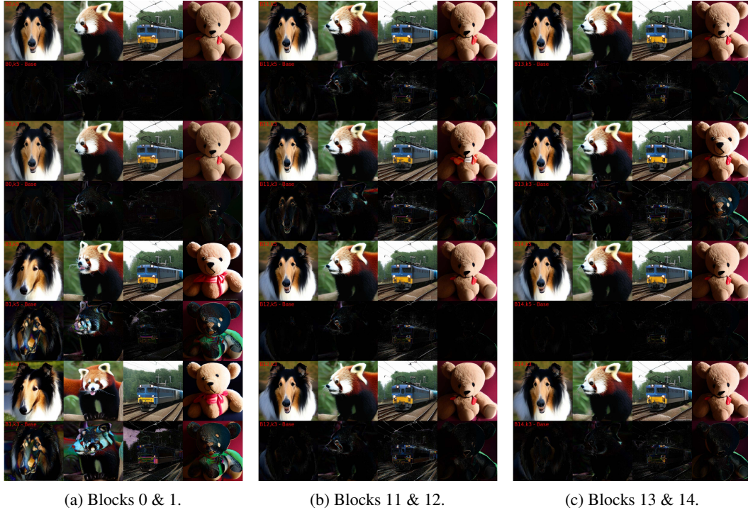
3756 Figure 91: Visual impact of adjusting the Natten kernel size for the outer blocks (independently). 3757 Block ID and kernel size is shown in the upper left corner in red text as "Bid,ksize", with k = 5 and 3758 k = 3 . Also showing deviations from the baseline case with k = 7 . Using 50 DDIM steps; cfg=4.
