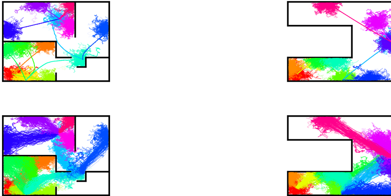
Figure 9: Difficulty of UPSIDE to cover the mazes if the hyperparameters T, H are set too large w.r.t. the environment size (here, T = H = 40 , and we recall that the mazes are of size 50 \times 50 ). Top (resp. bottom) row corresponds to the stochastic (resp. deterministic) executions of the policies of the directed parts of the skills.
