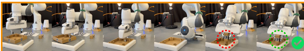
(D) Initial peg alignment is off, the policy corrects placement until it is properly inserted in the hole before letting go
