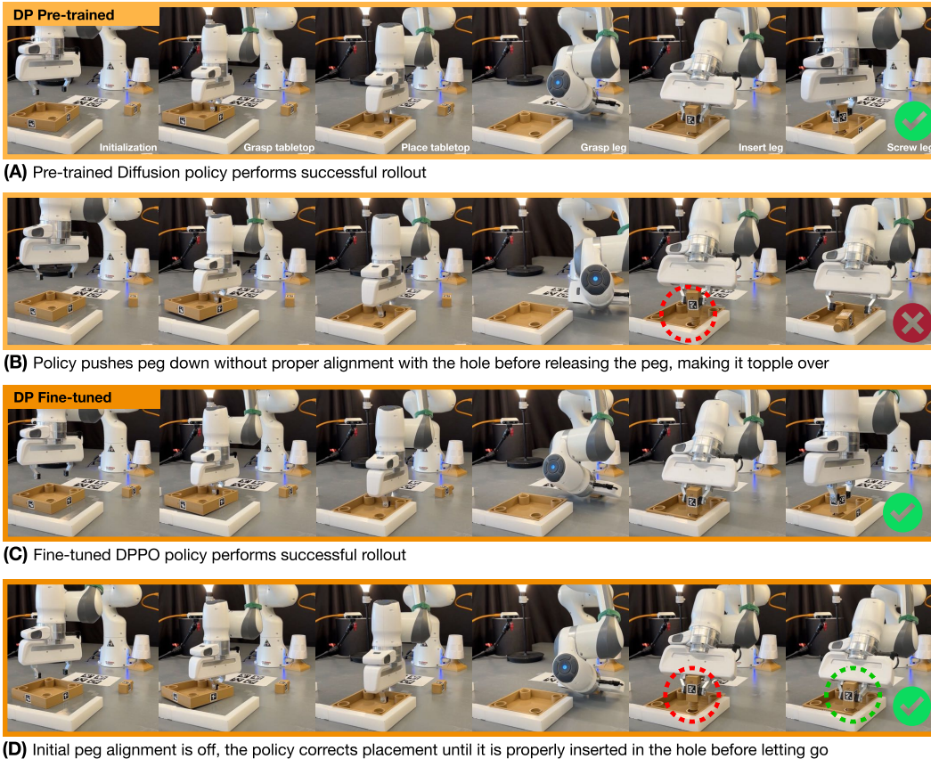
Figure 24: Qualitative comparison of pre-trained vs. fine-tuned DPPO policies in real evaluation. (A) Successful rollout with the pre-trained policy. (B) Failed rollout with the pre-trained policy due to imprecise insertion. (C) Successful rollout with the fine-tuned policy. (D) Successful rollout with the fine-tuned policy that requires corrective behavior.
