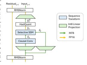
Figure 4: The precision mapping and dataflow of Quamba. All scaling factors and element-wise operations (*i.e.*, non-linearity and residual addition) are fused in the quantized operations.
