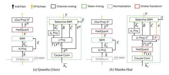
Figure 8: The figure compares Quamba to Mamba-Had. We fuse the Hadamard matrices in the linear layers to achieve compute-invariance.  $\overline{x}^p$  represents the 8-bit x tensor with percentile clipping. Our method provides real speedups on cloud and edge devices, while QuaRot requires extra Hadamard transforms and transpositions for SSM input activations. Residual connections are simplified to reduce clutter in the figure.
