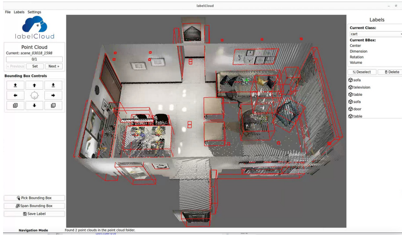
Figure 4: Example of object bounding box annotation.
