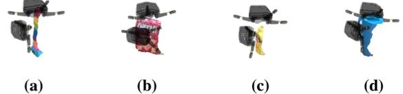
**Fig. 5:** MDN prior used for initialization, showing the top and side grasp modes for the partial view point clouds of the objects a lego blocks, b cracker box, c mustard bottle and d pitcher
